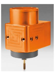
The moulding head transforms horizontal rotation into vertical rotation. The feed motion is carried out by a leader. The thread pitch of the leader corresponds to the pitch of the thread to be moulded. The moulding tool is operated with maximum precision with the help of the head spindle sleeve. A clamping sleeve is used to clamp the thread moulder.
