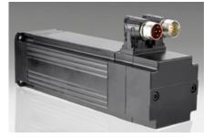
The drive consists of one synchronous servomotor for each moulding head that must be powered. The servomotor is configured according to the thread size. This makes it possible to create different thread sizes in a tool using one control. Thanks to the constant cutting speed, significantly longer service lives are achieved than is the case with mechanical, forced piloted systems. The drive is independent from the press stroke and press motion. The maximum rotation speed is 6000 U/min.
