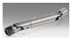
The drive shaft transfers the drive's torque to the moulding head. By evening out differences in height and length, the moulding head can be installed in every position within the tool. It is also manoeuvrable on holding-down plates. The maximum clearance between the drive and the moulding head is 500 mm.
